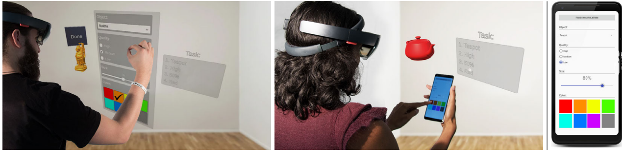
Figure 6: The conditions of the second experiment. Participants are either controlling the GUI via mid-air gestures (left), touch gestures on the smartphone or the GUI is displayed on the smartphone itself (center/right) while the task and elements are displayed in AR.
