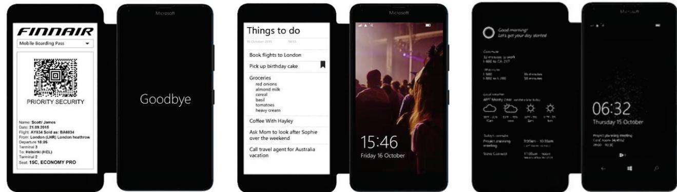
**Figure 3:** With our research concept, important information may be 'pinned' to the secondary display for instant, reliable access, e.g. e-tickets (which may be accessed even when the phone battery is depleted, left), to-do lists (middle) and a digital assistant (right). Manual 'pinning' of main display screenshots is supported by our prototype.
