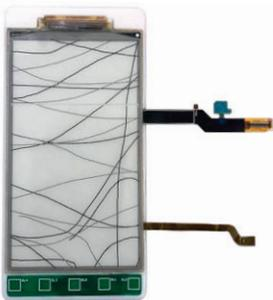
**Figure 2:** Between the grey soft-touch fabric which forms the display bezel and the Alcantara fabric on the outside of the cover, the e-ink display module and the touch buttons are mounted in a rigid 3D-printed housing to give the cover a uniform thickness (below).
