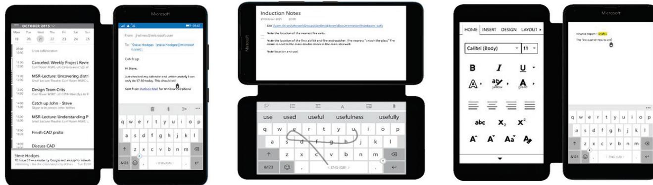
**Figure 4:** Our research concept can accommodate "laptop-class" tasks which require larger screen real estate than traditionally available on a smartphone. Examples include cross-referencing while authoring (left), a touch keyboard (middle) and a dual-screen application (right). In each case the e-ink Display Cover is used to extend the interaction surface. Note that these envisioned scenarios would require an e-ink touch overlay which our prototype does not have.
